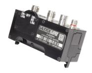
UHF SATCOM transmission - providing approximately 10dB of gain. A-320DPA works with AN/PRC-148, AN/PRC-152, AN/PRC-154 and MBITR II radios.
