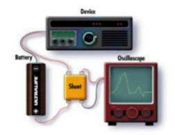
The setup of an oscilloscope and a shunt to monitor current requirements of a device.
